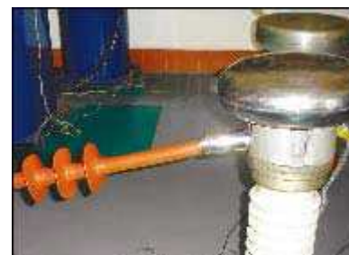
22kV 1-core outdoor termination is under testing
